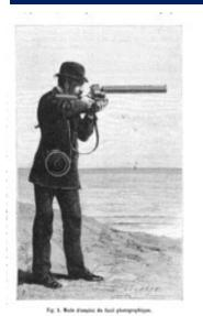
Rather than separate frames, Marey's "fusil photographique" allowed one to see motion continuously in a single static image.
