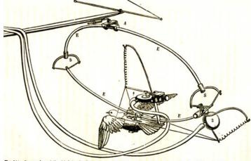
Fio. 104.—Suspension of the bird in the instrument. E E E E an ellipse of metal capable of oscillating freely in every direction, by means of the double suspension A. S S, india-nubber supports allowing the lower part of the ellipse to oscillate in the vertical direction. The suspensiony apparatus is fixed on the back of the pigcon. The leverdrum (i) receives the movements executed by the wing in a vertical direction. The lever-drum (2) receives those of the horizontal movements.
